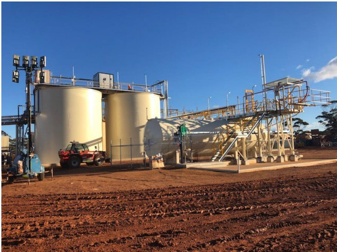
**Figure 1: Jaurdi Gold Processing Plant – Cyanide Facility and Leach Tanks**
