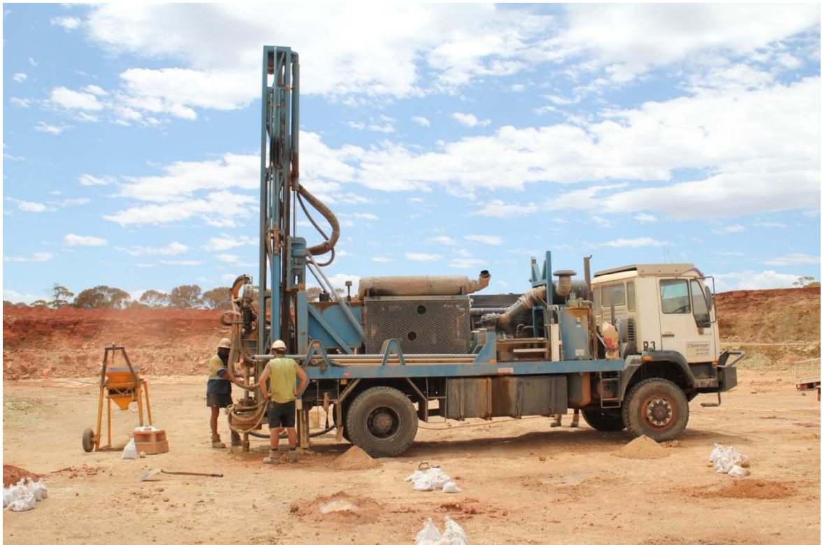
Grade control drilling on the pit floor
